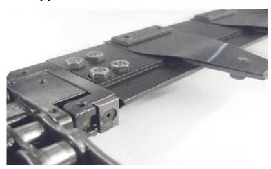
The grippers are made of special extra hard aluminum alloy, with anode treatment on the surface, ensuring accurate die cutting and embossing, ect. at high speed. The adjustment mechanism, patent design guarantees very accurate control. An imported chain is used for the main gripper transmission, with strength increased by 45% for accurate stability and prolonged life.
