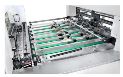
The incline-type paper moving table top is more suitable to high-speed thin paper and location. Side location adopt dual purpose side device with pull quide and push guide, accounting to paper choose, it makes switch easier. It could switch front rise position arriving reduction of speed device, it is benefit of thin paper's location.
