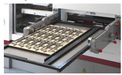
The driving gear ensures high speed of die cutting together. The pneumatic locking mechanism and air clutch are fast and stable. The die cutting frame can prevent the die cutting plate from drooping or separating effectively.
