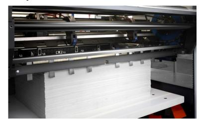
Delivery section add tester into security system. It is equipped with inset counter.
