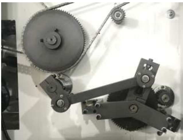
➤ Motor controlled gluing system. Inject glue and change the gluing sponge easily and quickly.
