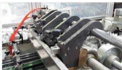
➤ Motor controlled gluing system. Inject glue and change the gluing sponge easily and quickly.
