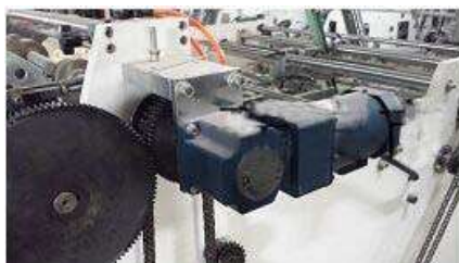
➤ Motor controlled gluing system. Inject glue and change the gluing sponge easily and quickly.
